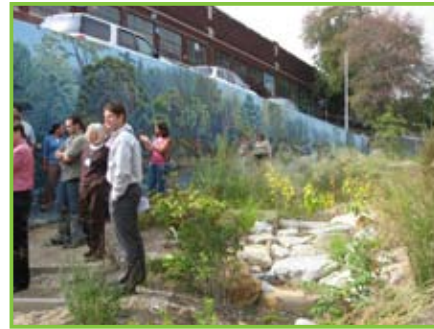
All of the stormwater runoff from the parking lot at Wissabickon Charter School in Philadelphia flows to a rain garden downhill from the school. The rain garden provides on-site educational opportunities at the school.
